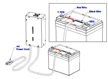
☐ When connecting two batteries in a series, it is imperative that the amount of charge and discharge be equal for both batteries. If there is an imbalance during charge or discharge, excessive battery voltage will occur. This will result in an overvoltaged battery and will cause dangerous battery out gassing and destruction. For accurate charge balancing, use one of our dual output chargers, such as the CT500 or TPRO series.
