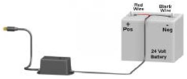
□ When connecting two batteries in series, it is imperative that the amount of charge and discharge be equal for both batteries. If there is an imbalance during charge or discharge, excessive battery voltage will occur. This results in an overvoltaged battery and will cause dangerous battery out gassing and destruction. For accurate charge balancing, use one of our dual output chargers such as the CT500 or TPRO series.
